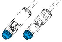
if the wiring is not needed. The puck is required for heat transfer, and will protect the fragile sample chamber pins at the bottom of the PPMS from damage.
