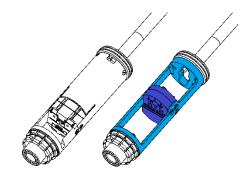
cell holder and the titanium cell does not distort the cell. The wiring needs to be fed through the holes in the top of the cell holder, the thermal link plate and the probe end plate.
