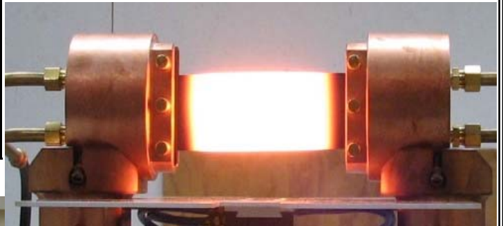
The flat plate assembly can be used up to 500 W/cm 2
