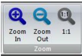
User can zoom-in or zoom-out the confocal image or color CCD image by this button. Note that it is a digital zoom, which changes the monitor display only and there is no change in FOV (field of view).
