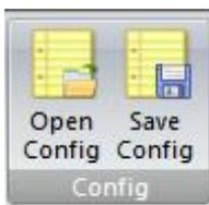
User can recall the control parameters used for the past works by Open Config, or save the current control parameters by Save Config. When the program starts, the default control parameters are called from the file **C:\ProgramFiles\Nanoscope Systems\NSWorks\config\DefaultParam.ini**.
