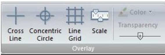
Some useful overlay can be showed on the live confocal image or color CCD image. It can be displayed on either display windows independently. The color and the transparency of the line can be adjusted for the current activated display window (confocal or CCD display window).
